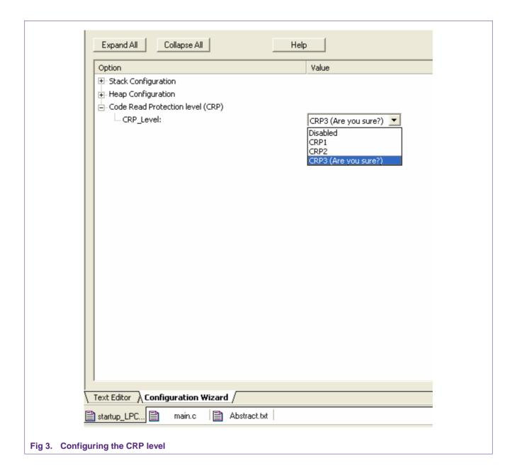
The *main.c* file contains additional modifications which allow breaking CRP3 using a hardware mechanism. In this example, we are using the central button of the Joystick (connected to P1.20) as the trigger to invoke boot loader in ISP mode. Please refer to Fig 3.
